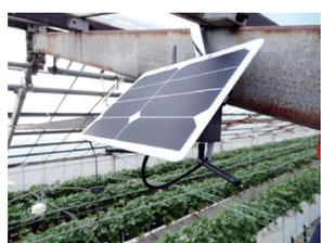
Sensor information such as soil moisture, temperature, humidity, soil PH · CO<sub>2</sub> can be viewed on the web. The web view provide means for storing Logs, data analysis and graphical presentation of real-time data.
